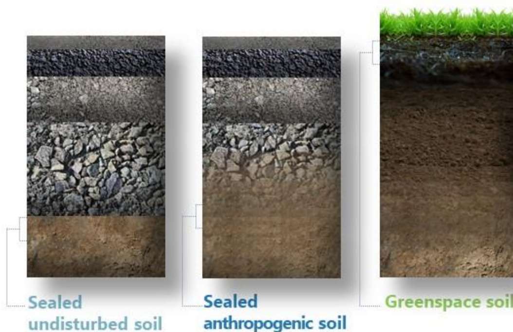
Figure 2: Diagram showing soil profiles and sampling depths of the three soil categories.
