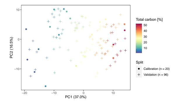
Figure 4. PC1 vs. PC2, computed via scaled and centered PCA, of the pre-processed local HAFL soil spectra (n = 116) colored by total carbon content [%]. The axis labels show the relative amount of variance explained [%] in parentheses. In this example, n = 20 representative samples were selected for calibrating a local model using the KS algorithm and the rest of the data were used for validation (n = 96).
