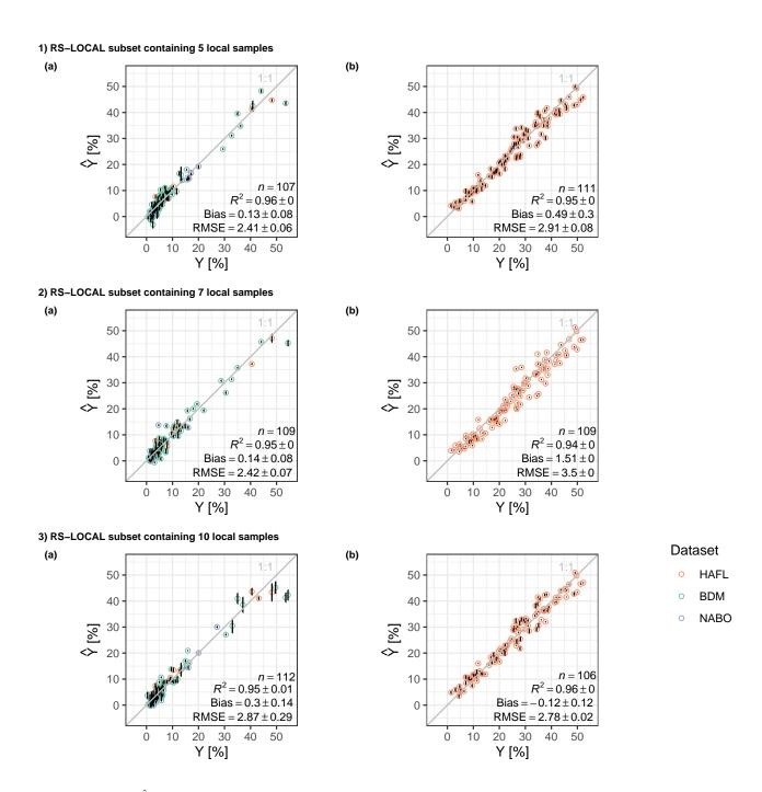
Figure 7. Predicted ( $\hat{Y}$ ) vs. observed (Y) total carbon content [%] by calibrating a PLSR of a RS-LOCAL subset with 5, 7 and 10 local HAFL samples (a) and validating it with the remaining local HAFL samples (n - 116) (b). The error bars signify the SD and where none are present, the components remained identical across 5 repeats and thus SD = 0.
