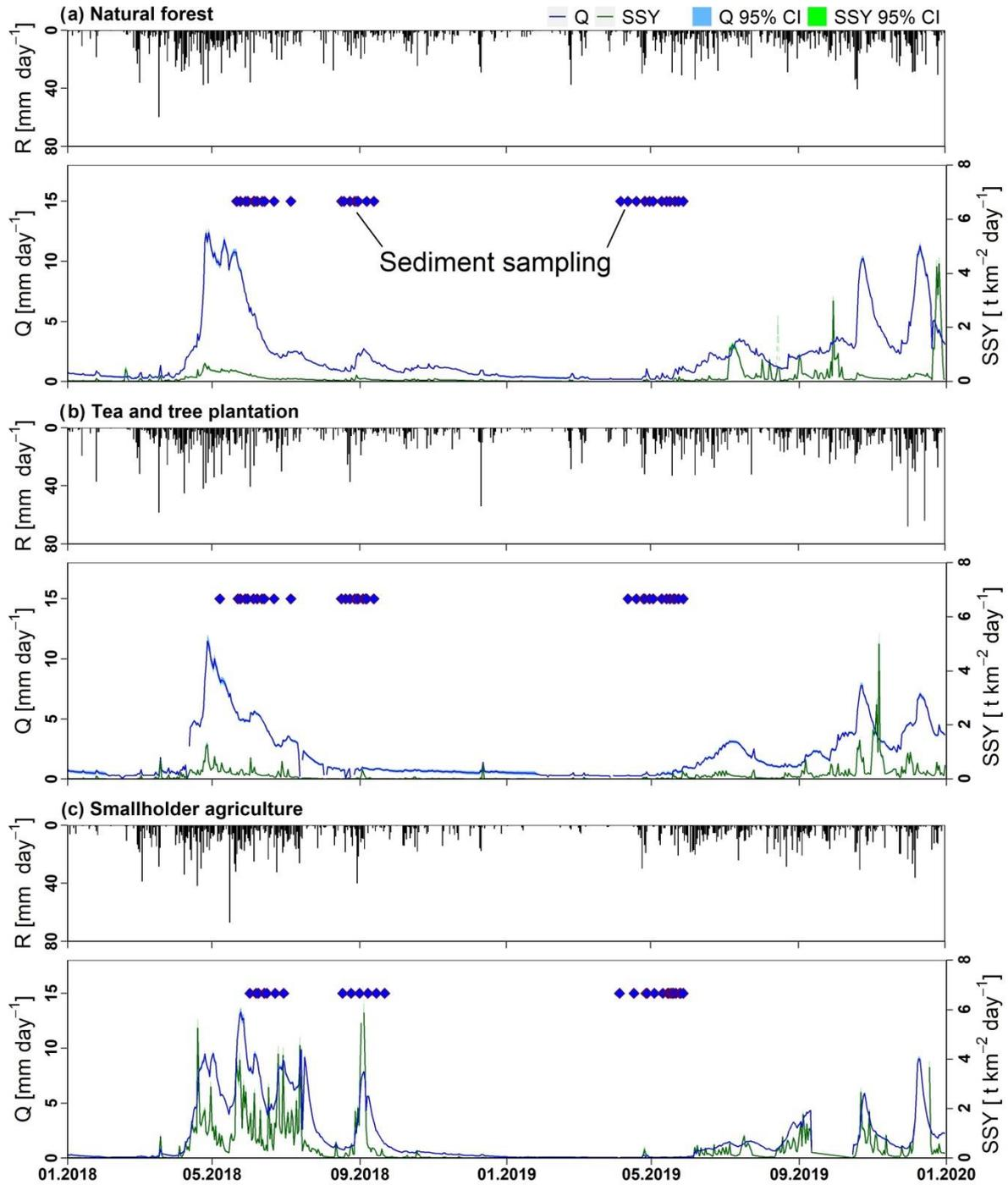
265 **Figure 3** Daily accumulated rainfall (R) [mm day<sup>-1</sup>], specific discharge (Q) [mm day<sup>-1</sup>] and suspended sediment yield (SSY) [t km<sup>-2</sup> day<sup>-1</sup>] aggregated from 10 minute resolution with 95 % confidence interval (CI) of the (a) natural forest, (b) smallholder agriculture and (c) tea-tree plantation catchments in the South-West Mau, Kenya between January 2018 and December 2019.
