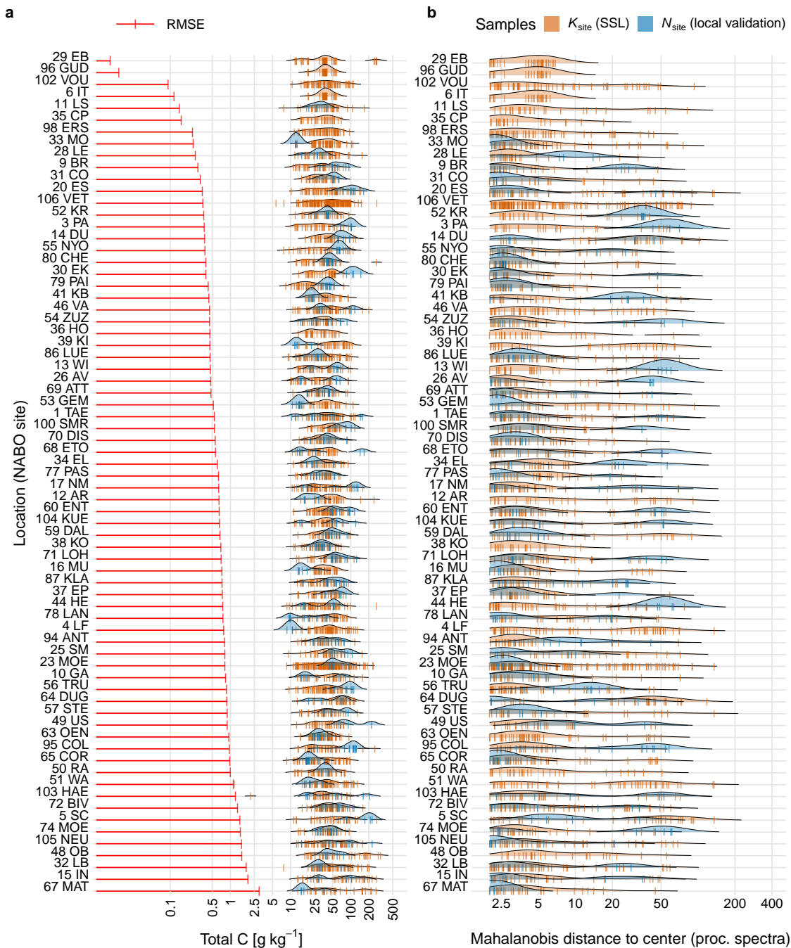
Figure 7. Analyzing the mechanisms behind the individual adaptive transfer realized with RS-LOCAL. Panel a : The left horizontal bars show the root mean square error (RMSE) of mid-infrared predictions of the temporal validation set N_{\text{site}} of time series of total carbon (C) for each of the 71 NABO sites, which was calculated without the two respective calibration samples. The blue density plots depict the distribution of the site-specific validation samples, and the brown vertical bars show the measured values of C for the final subsets of SSL used for the transfer ( K_{\text{site}} ). Panel b : The distribution of the robust distances from the PCA center of Savitzky-Golay preprocessed spectra of the entire soil spectral library compared to the subset of instances involved in the individual transfer modeling ( K_{\text{site}} ) and validation samples ( N_{\text{site}} ) (similarity in site-specific vs. final RS-LOCAL selection), computed with the Minimum Covariance Determinant (MCD) estimator.
