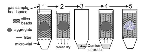
**Figure 1.** Schematic diagram showing a series of five steps in the treatment of the aggregates in their vials: 1) headspace gas removal, 2) freeze-drying, 3) & 4) staining with  $OsO_4$  and 5) scanning in the synchrotron beamline.
