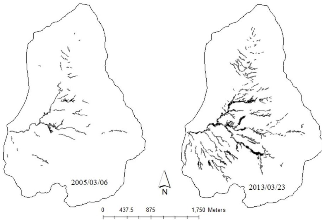
720 Fig. 3. Gully drainage network expansion in the Debre Mawi watershed, Ethiopia, between 2005 and 2013. Lines represent gully
