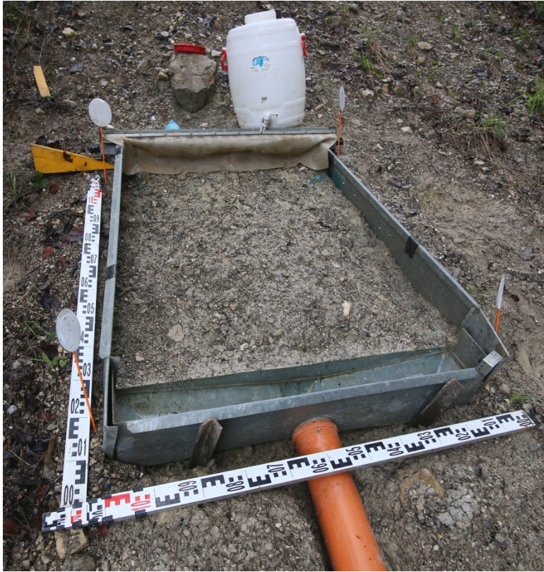
3 Figure 1. Experimental setup including plot, 30 litre barrel, runoff collector, reflectors for 4 tachymeter registration and measuring stick for scaling purposes
