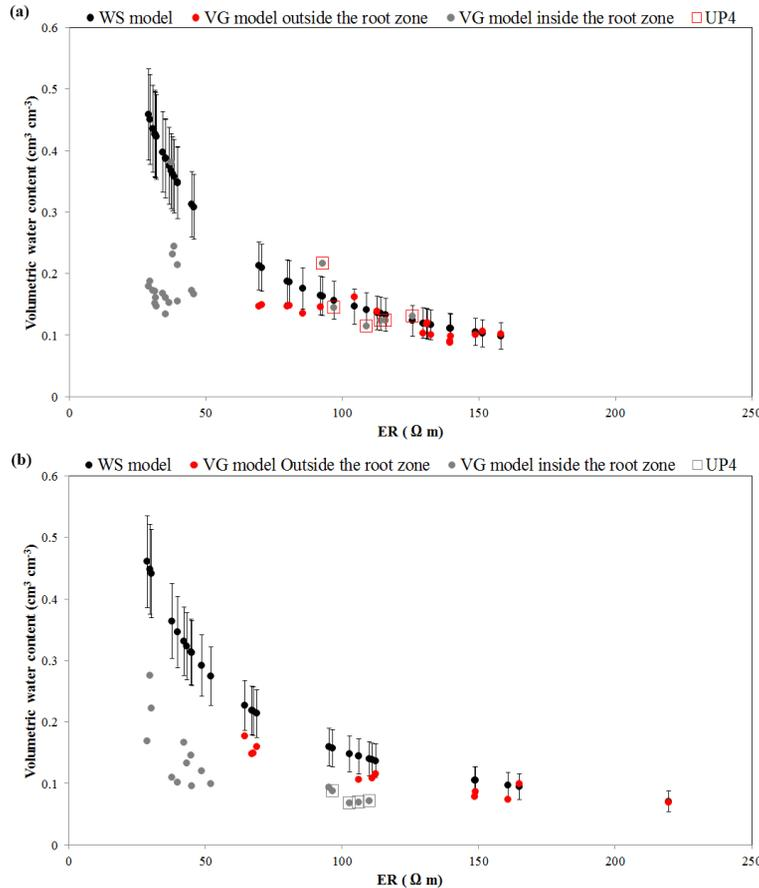
**Figure 8.** Relationship between VWC and ER in the top soil for the wet period (T01 to T06) **(a)** and the dry period (T07 to T10) **(b)**. Black circles with standard deviation indicate VWC from Waxman and Smits model. Red and grey circles indicate VWC predicted from retention curve respectively outside and inside the root zone.
