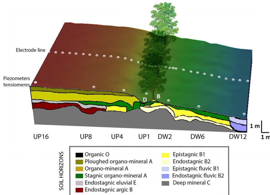
**Figure 1.** Experimental setup and soil cross section. Soil was excavated up along the toposequence from 16 m upslope (UP16) to 12 m downslope (DW12). Soil horizons are named according to the *World Reference Base for Soil Resources* (FAO, 1998). D and B indicate respectively ditch and bank locations. Each monitored location at UP16, UP8, UP4, UP1, DW2, DW6 and DW12 was equipped with 5 tensiometers and 1 piezometer.
