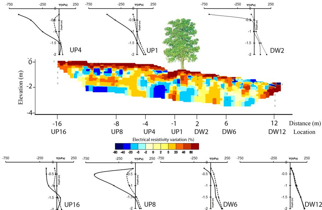
**Figure 5.** ER variation (%) from initial wet state (T06) to the final dry state (T10) compared to measured soil matric potential profiles. 7 locations i.e. UP16, UP8, UP4 and UP01 for upslope and DW2, DW6 and DW12 for downslope were monitored. The dashed lines indicates the initial wet state and solid lines the final dry state.
