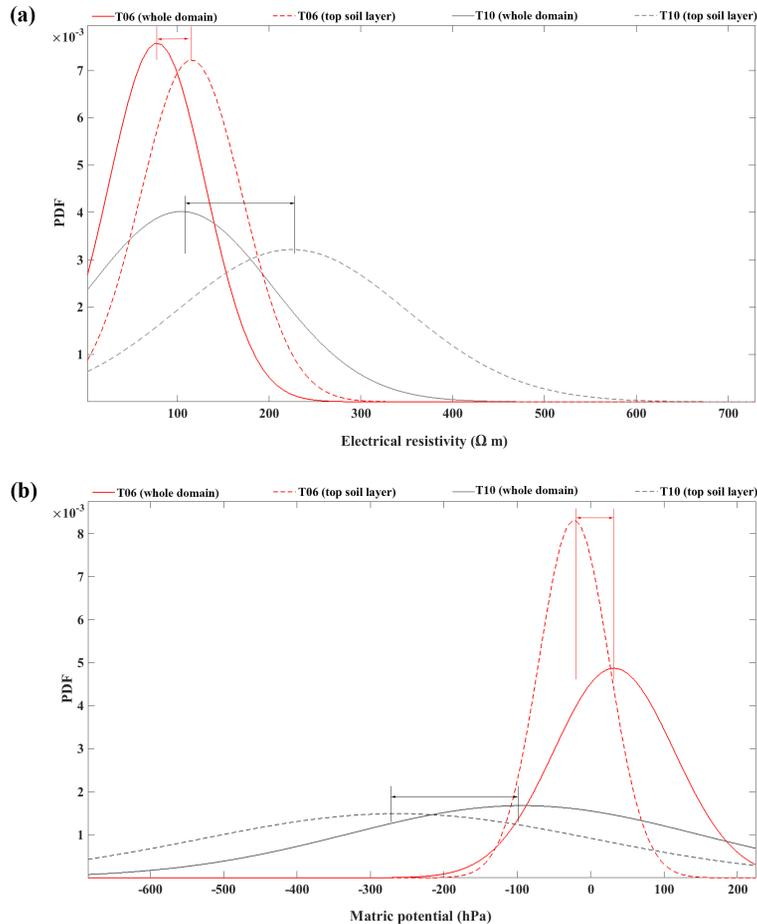
**Figure 6.** Probability density functions (PDF) of **(a)** electrical resistivity and **(b)** matric potential between wet (T06) and dry (T10) states for the whole domain (solid line) and for the topsoil layer (dash line).
