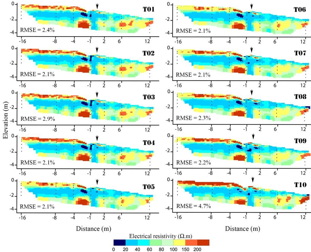
**Figure 4.** ERT maps at 10 measurement dates (from T01 to T10). Black points indicate tensiometer locations and black arrow the hedgerow location.
