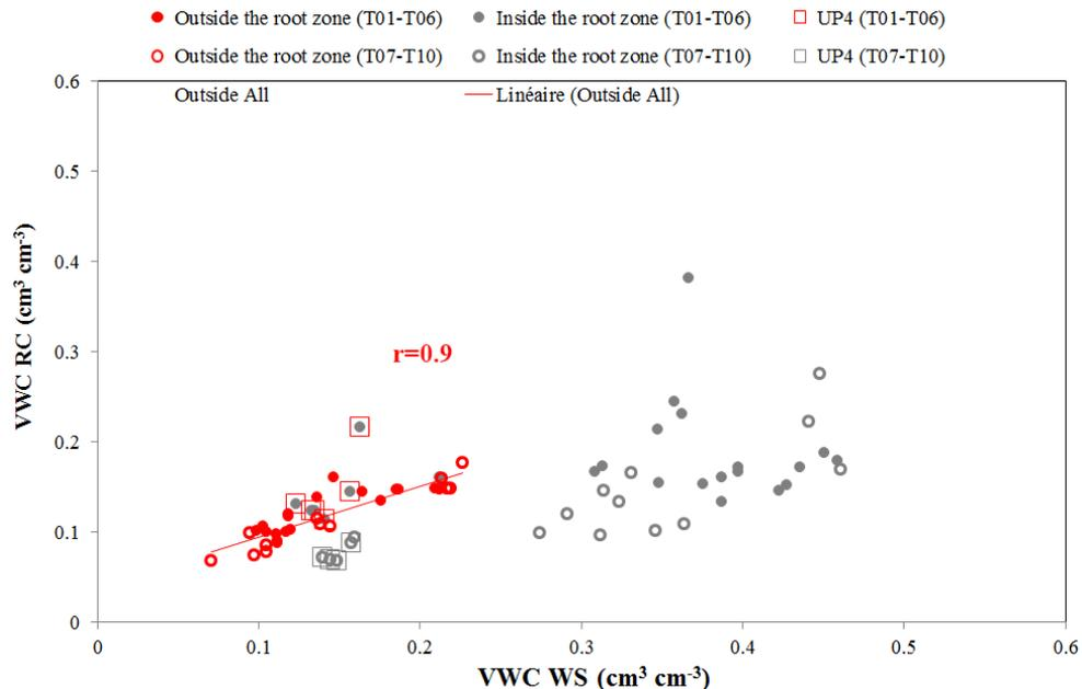
**Figure 9.** VWC from Waxman and Smits model compared to retention curve prediction outside the root zone (red circles) and inside the root zone (grey circles). The full circles represent the wet period (T01 to T06) and the open circles the dry period (T07–T10).
