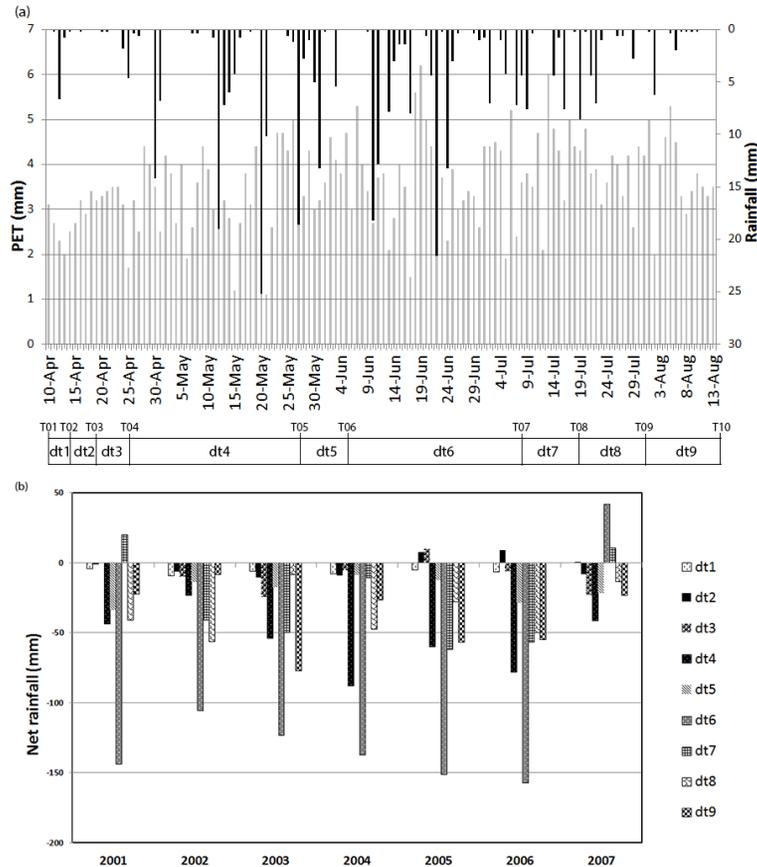
**Figure 2.** (a) Daily rainfall and potential evapotranspiration (PET) measured during the monitoring period (10 April to 13 August 2007). ERT measurement dates (T01 to T10) and intervals between them (dt1 to dt10) are indicated along the x axis. (b) Net rainfall (rainfall – PET) calculated for each interval of the monitoring period and compared to those of the previous 6 years.
