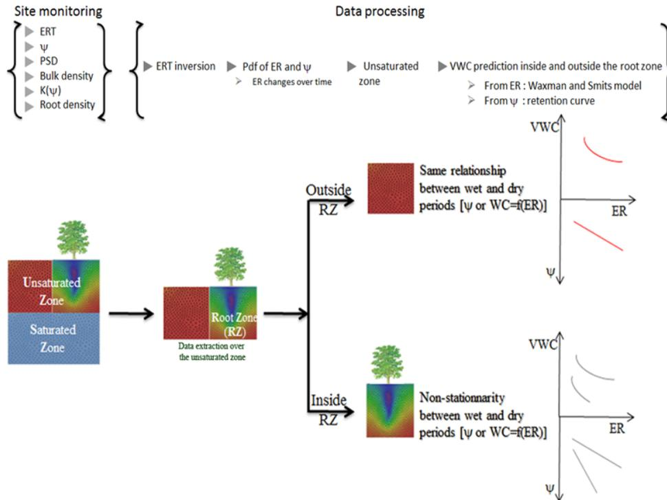
**Figure 10.** Conceptual scheme summarizing the methodology from site monitoring to data processing.
