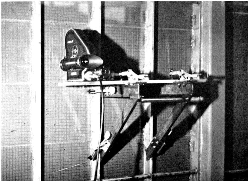
**Figure 15.** Time-lapse photography set-up used by Klepper and Huck at the Auburn Rhizotron to examine root behavior behind glass panels (Courtesy of Alabama Agricultural Experiment Station). The camera support could be moved to allow photography of any part of the visible root system. The 1/2 inch square grid-wire mesh embedded in the glass panes provided a measuring scale and reduce shattering if the glass broke (from Taylor, 1969).
