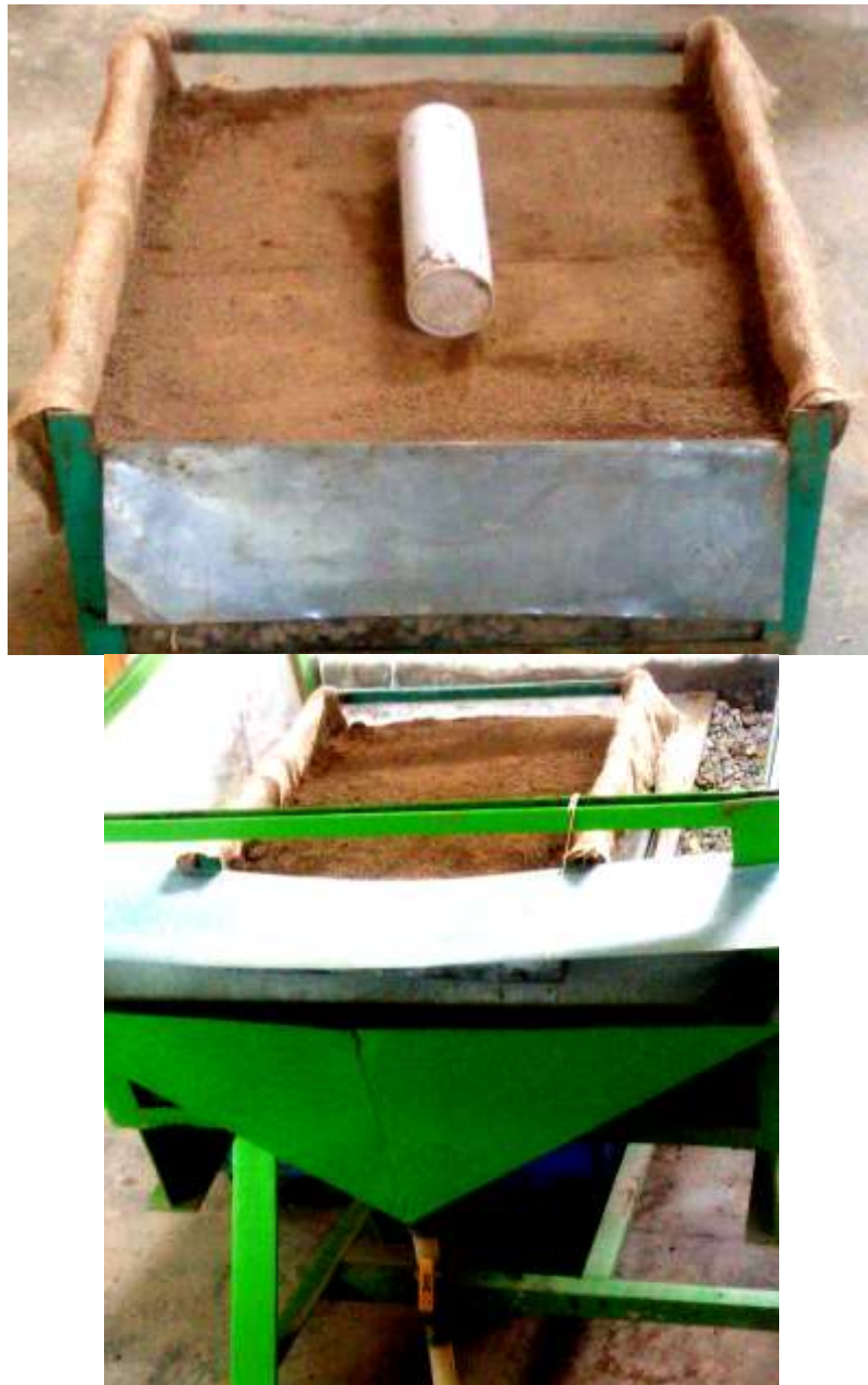
Figure 1. A general view of the experimental setup at Rainfall and Soil erosion Simulation Laboratory of Tarbiat Modares University, Iran
