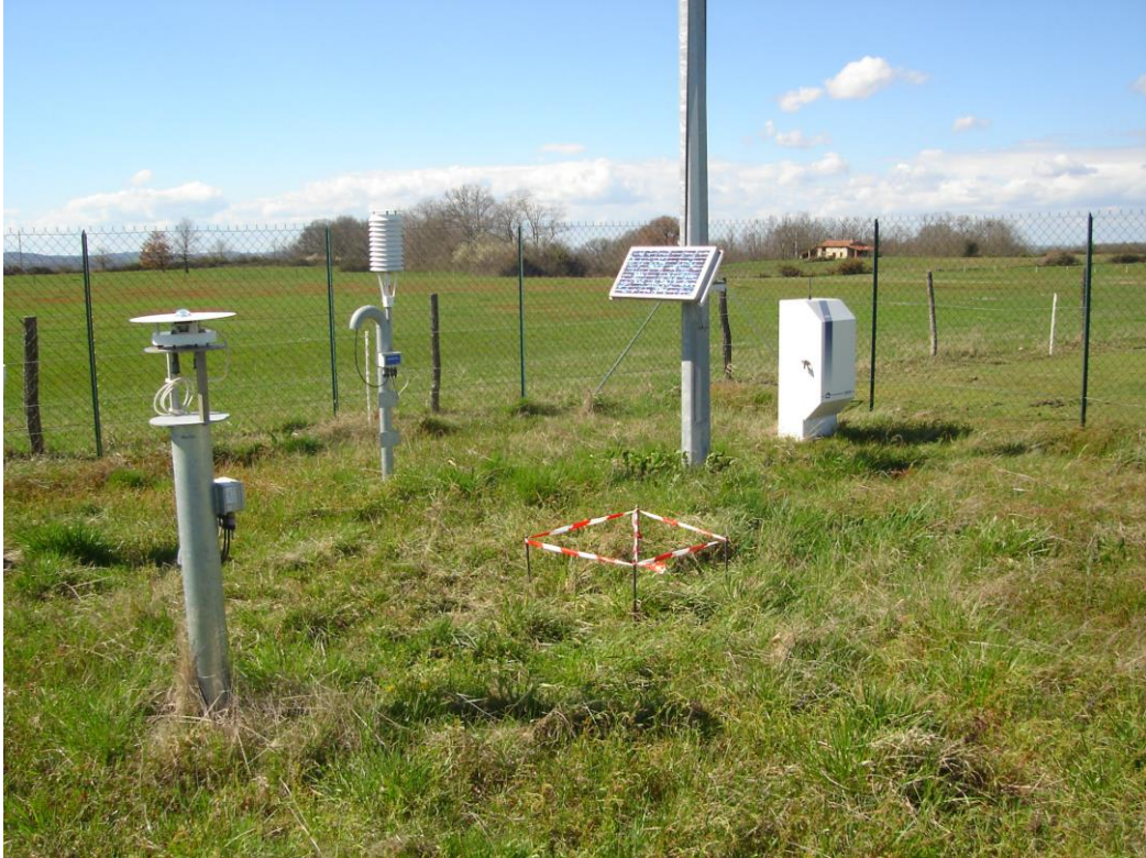
Figure S1.4 - Automatic weather station of Montaut (MNT).
