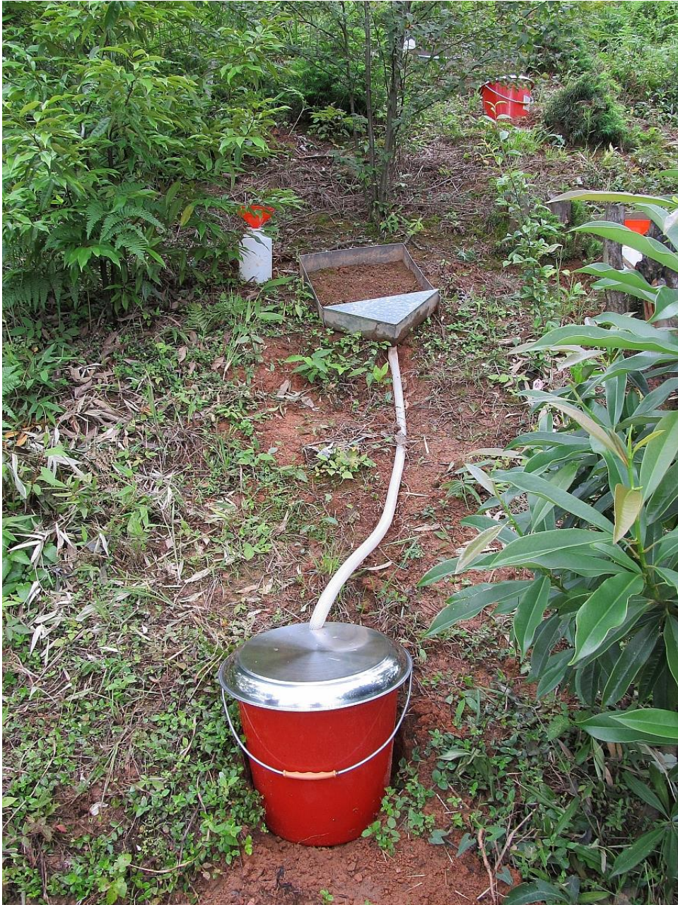
812 Figure 1: Measurement setup showing a runoff plot (ROP, 0.4 m × 0.4 m) with reservoir and rainfall gauge on the 813 experimental site in Xingangshan, Jiangxi Province, PR China.
