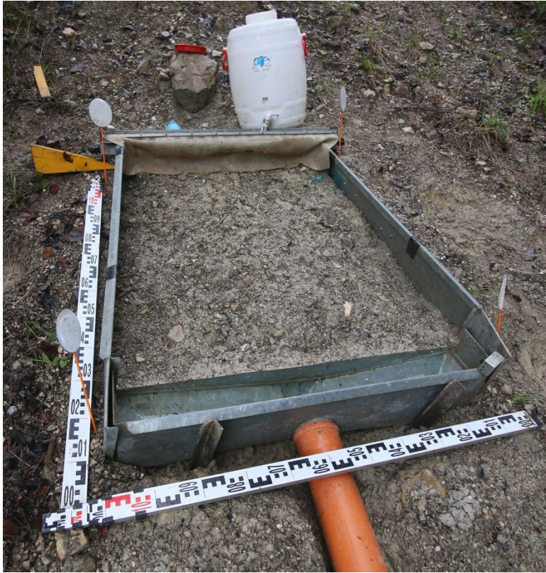
Figure 1. Experimental setup including plot, 30 litre barrel, runoff collector, reflectors for tachymeter registration and measuring stick for scaling purposes
