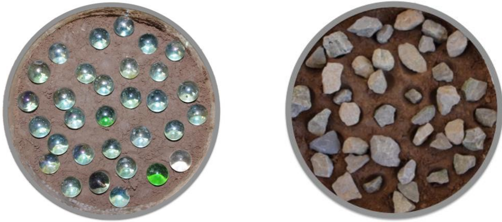
Fig. 1 – Preparation of disturbed samples containing glass balls (left) and gravels (right).
