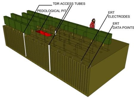
**Figure 1.** Scheme in 3D which illustrates the equipment of the experimental plot in the vineyard with devices for hydric and geophysical field-data acquisition. This image already appeared in Brillante et al. 2014, courtesy of Elsevier.
