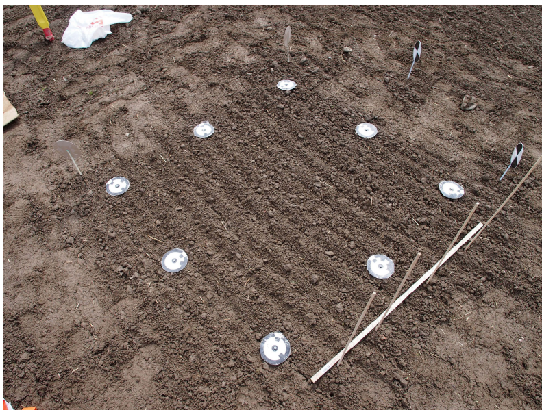
Figure 2. Setup of the measurement plot. The markers delineate an area of 1\text{ m}^2 . The patterns on the markers were used for the stereophoto technique.
