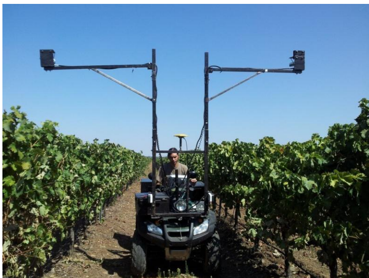
Figure 3. ATV with two multi-spectral sensors for NDVI mapping of vineyard canopy
