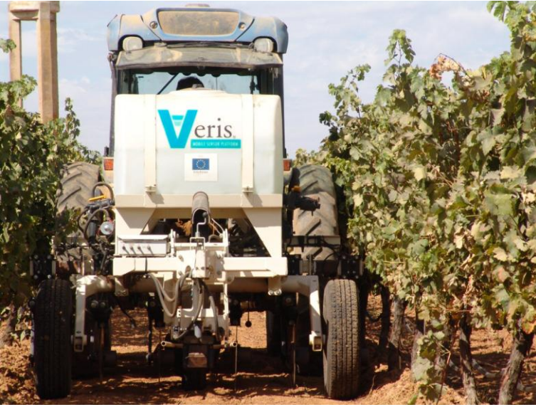
Figure 4. Mobile sensor platform Veris 3150 for ECa mapping.
