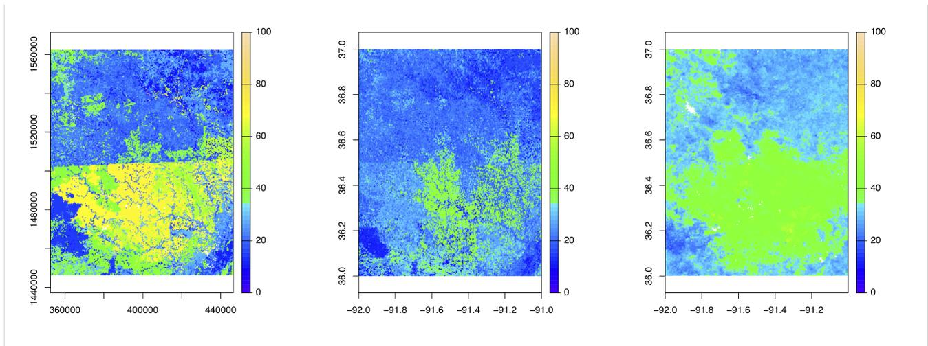
**Figure S2.** Maps of clay concentration % in the 30-60 cm depth slice, Missouri-Arkansas border; lower-right corner near Pocahontas AR. (left) gNATSGO; (center) PSP; (right) SG2
