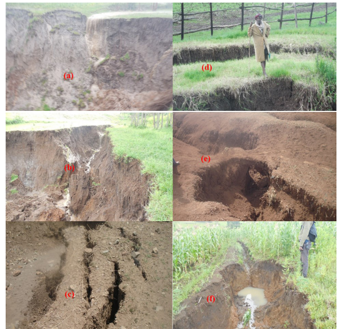
Figure 1. Examples of gully expansion controlled by (a, b) bank geometry (height and slope), (c) tension cracks, (d) landslide, (e) soil pipes, and (f) saturated Vertisols (gully development on conservation ditches, narrow ditch upstream of gully headcut in the subhumid Debre Mawi (a, b, d, f), Mota (c), and Geregera (e) watersheds (pictures taken in 2013).
