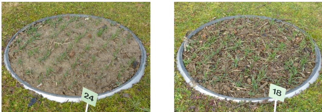
Figure B2. Lysimeter with winter wheat under conventional tillage (CT, left) and under non-inversion tillage (NIT, right) treatment on 14 January 2016.
