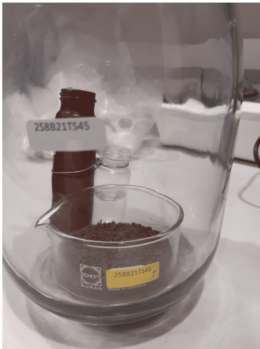
Figure S1. Incubation setup: A 2-l glass jar containing a Petri dish filled with 50 g of soil material, a brown vial containing NaOH solution to trap the respired CO 2 and a smaller clear vial containing water to keep a constant humidity within the jar.
