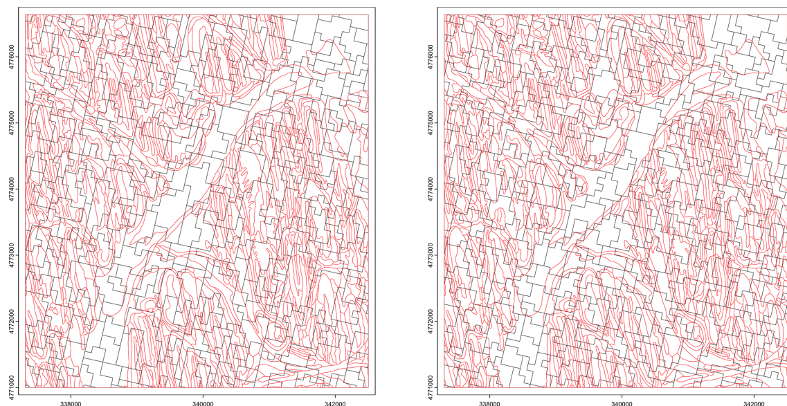
Figure 27. Supercells derived from the clay concentration % of the 0–5 cm layer from SOLUS 100 m overlaid by the polygon boundaries (in red) from gSSURGO. Compactness parameter 0.2 (left), 2.0 (right). Projection is UTM18N on WGS84, compare with Fig. 25.
