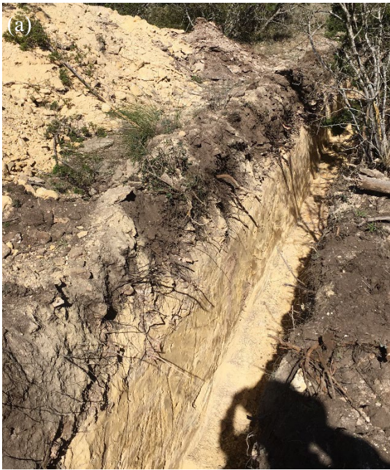
Figure S3. Trench 5A (a) and Trench 6 (b) in Buda soil at Texas A&M AgriLife Sonora Research Station on the Edwards Plateau, Texas. The yellow-whitish layer of Trench 5 is unconsolidated paralithic (Cr) layer weathered from limestone. The gray fractured layer between A and Cr horizons in Trench 6 is petrocalcic (Bkkm) horizon.
