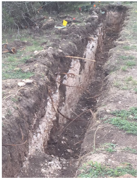
Figure S3. Trench 5A (a) and Trench 6 (b) in Buda soil at Texas A&M AgriLife Sonora Research Station on the Edwards Plateau, Texas. The yellow-whitish layer of Trench 5 is unconsolidated paralithic (Cr) layer weathered from limestone. The gray fractured layer between A and Cr horizons in Trench 6 is petrocalcic (Bkkm) horizon.
