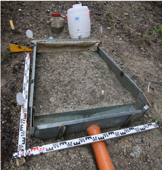
Figure 1. Experimental setup including plot, 30L barrel, runoff collector, reflectors for tachymeter registration and measuring stick for scaling purposes.
